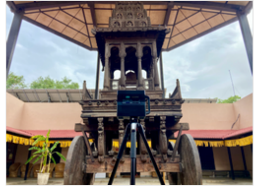
A structured-light 3D scanner (Matterport Pro2) creating a digital twin of a historic temple chariot at the National Crafts Museum, Delhi.
